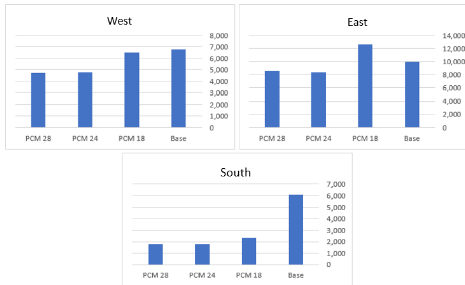
Fig 9: Comparison of energy consumption in the basic state and with PCM in the investigated directions during the year.
